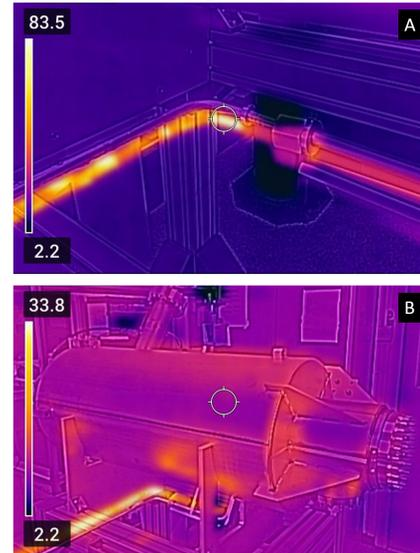
Figure 4: Thermal imaging of A, the helium jacket inlet, and B, the cavity helium jacket.
