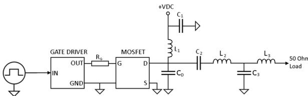
Figure 6: RF circuitry of the Class-E 1 kW module.
