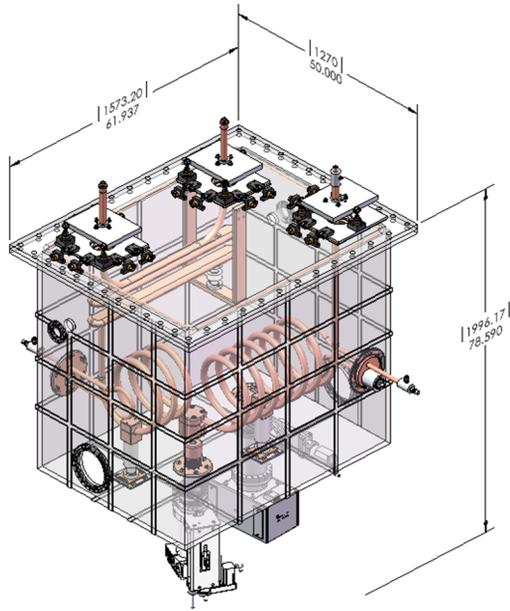
Figure 5: Engineering design of the RF sweeper with overall dimensions in millimeters (in brackets) and inches.
