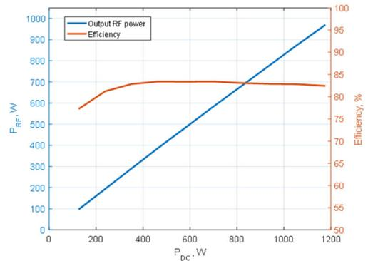
Figure 7: Measured output RF power and efficiency vs. DC power for the 1 kW module.
