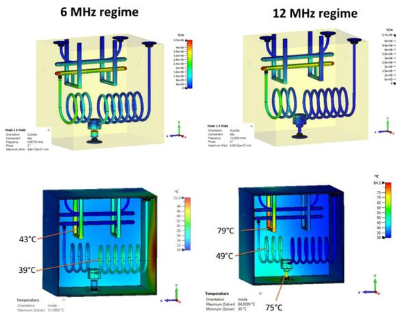
Figure 3: The surface electric fields in the sweeper (top) and the thermal maps (bottom) for 6 MHz and 12 MHz regimes normalized to 1 J.
