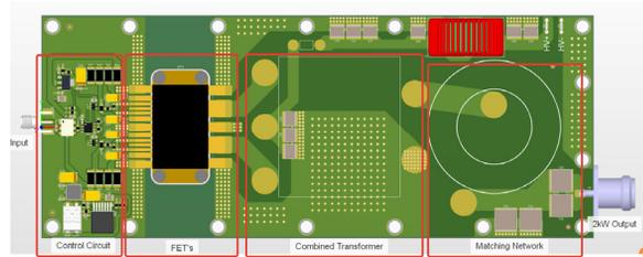
Figure 8: Amplifier pallet design of the 2-kW module.
