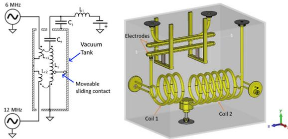
Figure 2: Schematics of dual frequency RF sweeper (left) and its 3D model (right).
