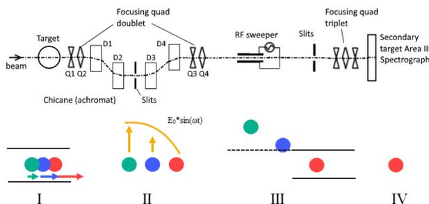
Figure 1: Layout of the ATLAS in-flight RIB facility (top) and the scheme of rare isotope RF separation (bottom).
