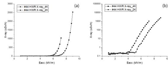
Figure 4: Turn-on  $E_{acc}$  of x-ray radiation of No.44 HWR: the square line and the circle line represent 4K and 2K x-ray radiation, respectively, (a) plotted in linear scale and (b) replotted in log scale.
