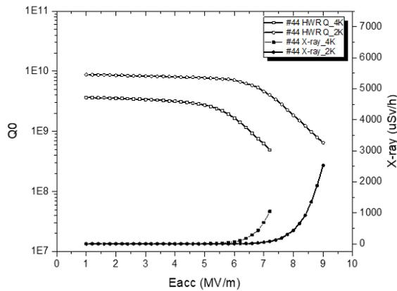
Figure 1: Quality factor and x-ray radiation of No.44 HWR: the square line and circle line represent 4K and 2K data, respectively.
