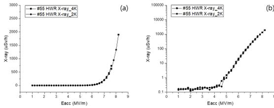
Figure 6: Turn-on  $E_{acc}$  of x-ray radiation of No.55 HWR: the square line and the circle line represent 4K and 2K x-ray radiation, respectively, (a) plotted in linear scale and (b) replotted in log scale.
