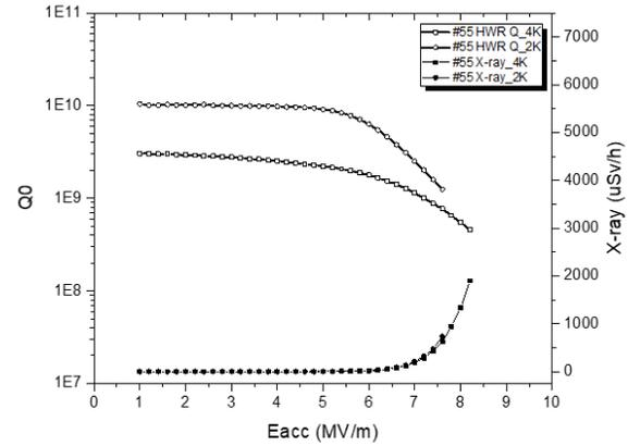
Figure 3: Quality factor and x-ray radiation of No.55 HWR: the square line and circle line represent 4K and 2K data, respectively.
