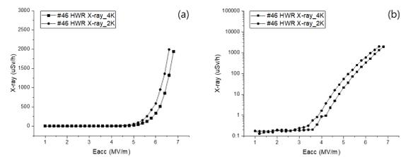
Figure 5: Turn-on  $E_{acc}$  of x-ray radiation of No.46 HWR: the square line and the circle line represent 4K and 2K x-ray radiation, respectively, (a) plotted in linear scale and (b) replotted in log scale.
