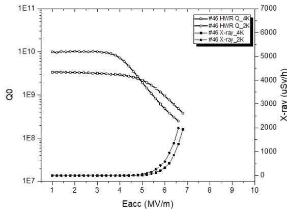
Figure 2: Quality factor and x-ray radiation of No.46 HWR: the square line and circle line represent 4K and 2K data, respectively.
