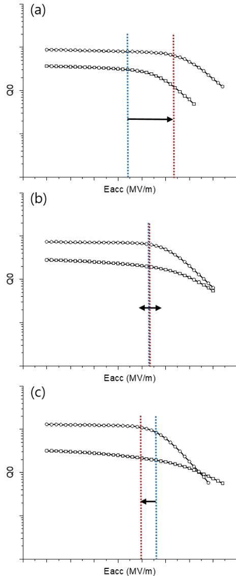
Figure 7: Three types of Q-drop tendencies with FE conditioning: (a)  $\beta_{2K} < \beta_{4K}$ , turn-on  $E_{acc,ON}$  increased, (b)  $\beta_{2K} \sim \beta_{4K}$ , turn-on  $E_{acc,ON}$  remains almost same, (c)  $\beta_{2K} > \beta_{4K}$ , turn-on  $E_{acc,ON}$  decreased.
