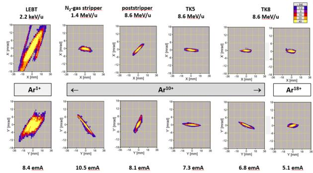
Figure 5: High intensity  $^{40}\text{Ar}$ -beam emittance and current measurements along UNILAC and TK.
