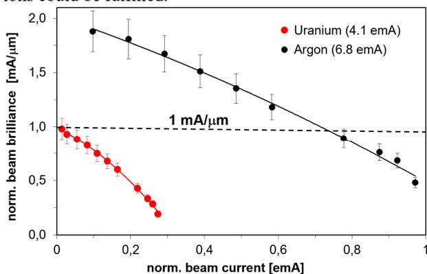
Figure 7: Normalized  $\text{Ar}^{10+}$  and  $\text{U}^{28+}$  (fractional) beam brilliance analysis based on beam emittance and corresponding beam intensity measurements at the end of the transfer line (TK8) to the SIS18; The data refers to the normalized high current FAIR requirement of  $1\text{ mA}/\mu\text{m}$  defined for  $\text{U}^{28+}$  as reference ion ( $A/Z = 8.5$ ;  $I = 15\text{ eA}$ , hor. emittance =  $1\ \mu\text{m}$ ).
