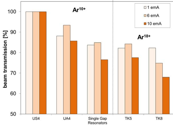
Figure 3: Beam transmission at poststripper and transfer line to SIS18 for different beam currents.
