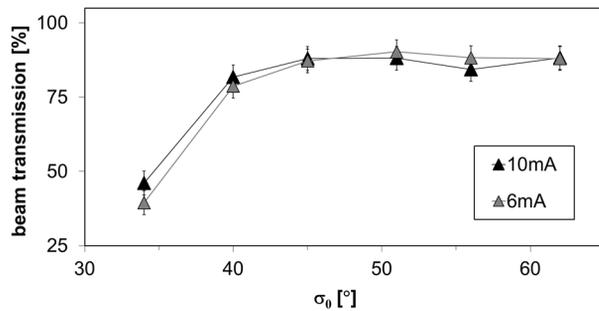
Figure 4:  $\text{Ar}^{10+}$ - beam transmission as function of the zero current phase advance for two different beam currents.
