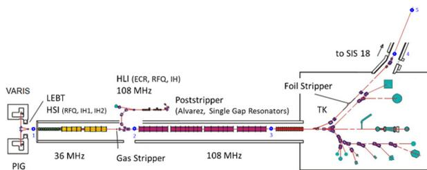
Figure 1: GSI-UNiversal Linear ACcelerator (UNILAC); the slit-grid-emittance measuring devices are shown in blue; 1: LEBT/UH1, 2: gas stripper section/US4, 3: poststripper/UA4, 4: transfer line/TK5, 5: transfer line/TK8.
