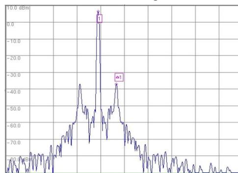
Figure 5: Spectral analysis of the master oscillator driver, with 1 Hz resolution and video bandwidths.
