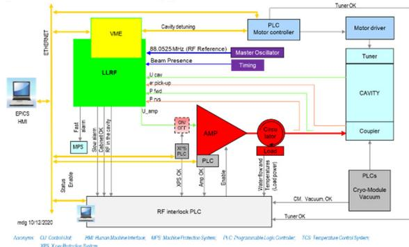
Figure 1: SC cavity RF system block diagram.
