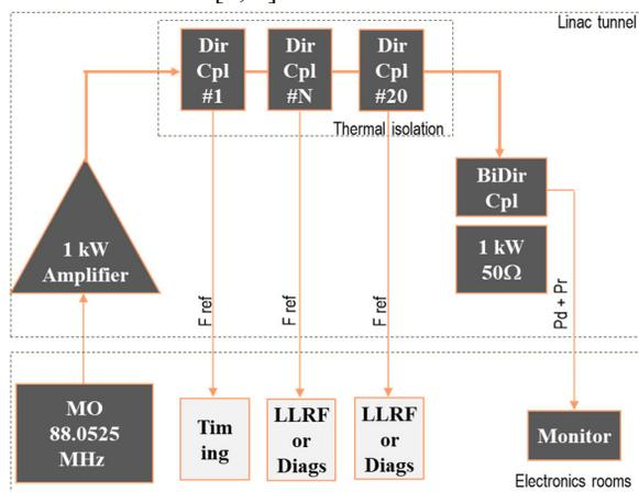
Figure 4: MO and reference distribution bloc diagram.
