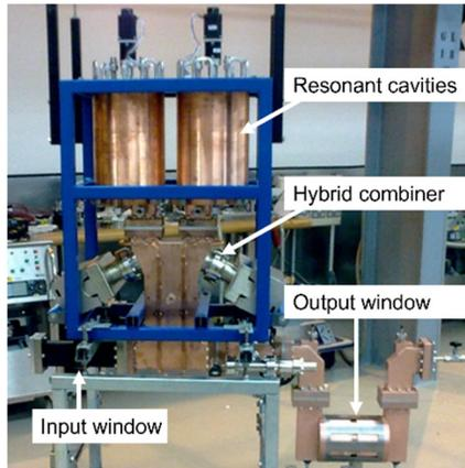
Figure 3: SLED cavity assembly.
