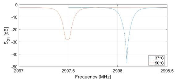
Figure 6: Thermal tuning of SLED cavity.
