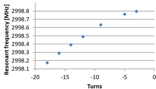
Figure 5: Mechanical tuning of SLED cavity.
