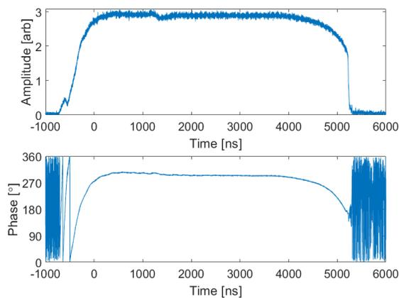
Figure 8: Klystron output with square drive.
