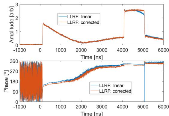
Figure 10: SLED output with empirical LLRF tuning.
