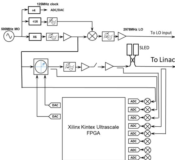
Figure 4: Low level RF schematic.
