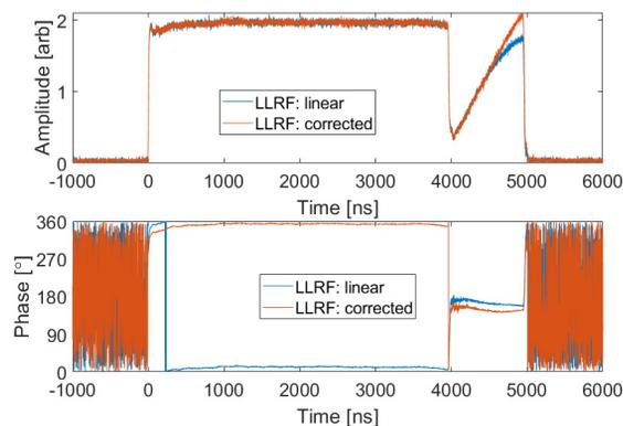
Figure 9: Klystron output with empirical LLRF tuning.
