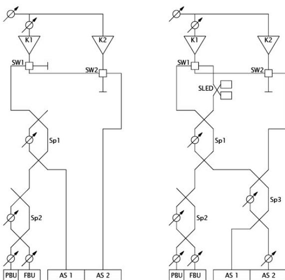
Figure 1: Linac configuration without (left) and with (right) SLED cavity.
