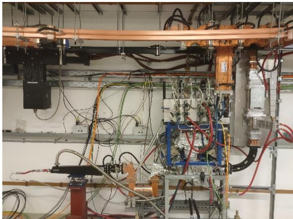
Figure 7: Installation for high power test into water load.
