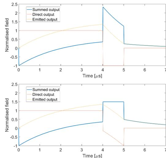
Figure 2: Calculated SLED performance with phase flip (above) and additional amplitude shaping (below).
