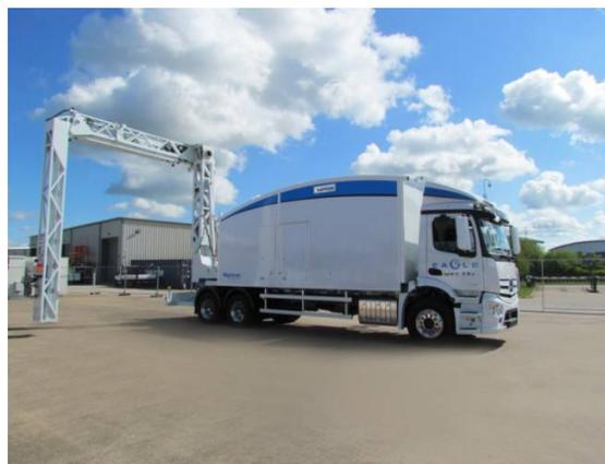
Figure 1: Rapiscan Eagle M60 in the deployed position ready for scanning.
