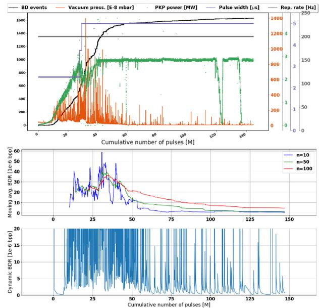
Figure 4: Full conditioning history of one LIGHT accelerating cavity. The top picture shows the cumulative number of breakdowns, the pulse width, the repetition rate, the RF power, and the vacuum pressure across the cumulative number of RF pulses. The bottom picture shows the BDR moving average and the dynamic BDR across the cumulative number of RF pulses.
