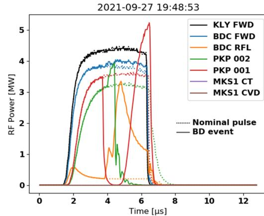
Figure 3: Example of acquired signals. Breakdown event in solid lines and previous nominal pulse in dotted lines.
