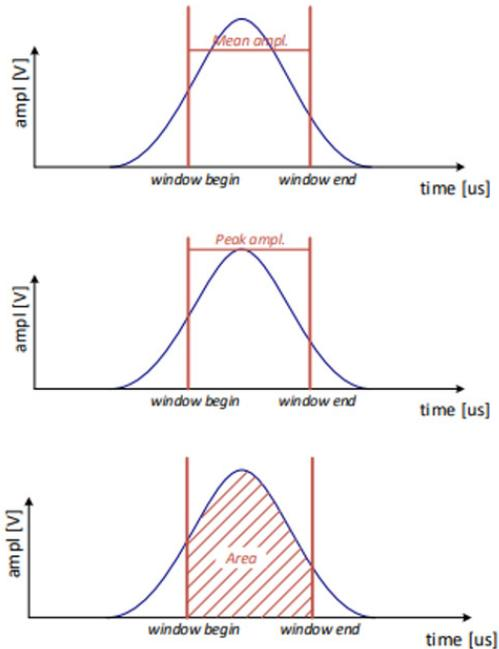
Figure 2: Sketch of the three types of measurements applicable to the acquired signals.
