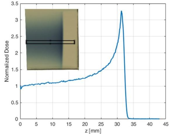
Figure 4: Bragg peak measured at beam output using EBT3 radiochromic film. The z-coordinate corresponds to the penetration depth in water.
