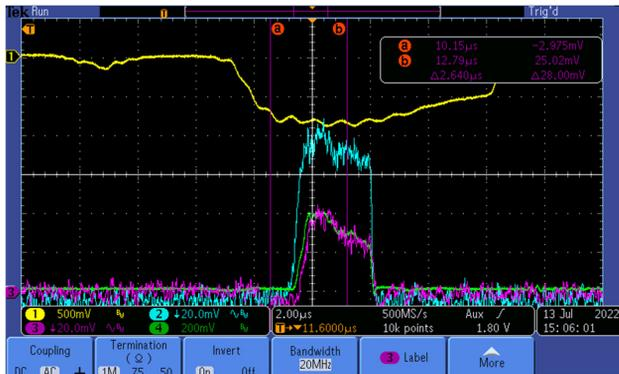
Figure 3: Screen image of the 63 MeV acceleration.
