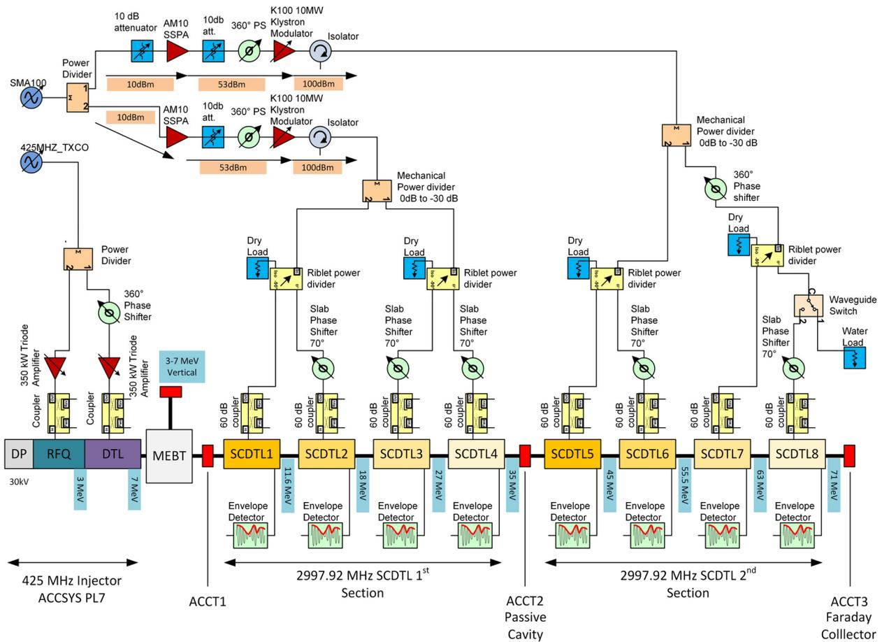
Figure 2: TOP-IMPLART linac schematic representation showing RF distribution network and beam diagnostics.
