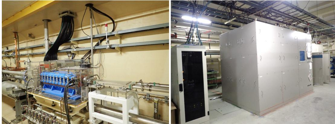
PF pulsed bending magnet and pulsed power supply
