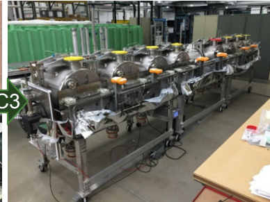
Cold mass ready for baseplate
