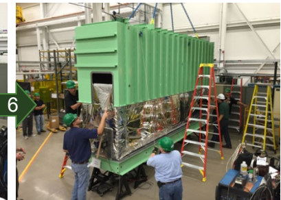
Vessel cover installation
