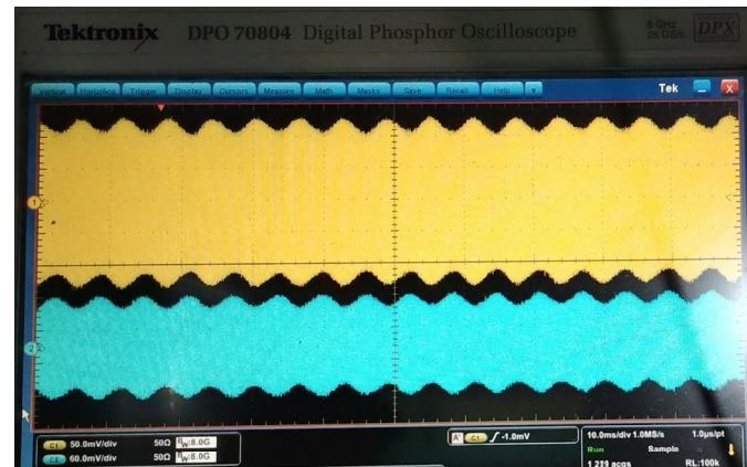
Spontaneous Amplitude Modulation of the two EACA cavities in anti-phase, above a 12 MV/m (total gradient) threshold.
