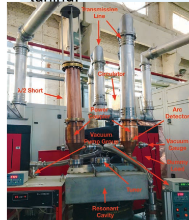
4616V4 tetrode amplifiers commissioned: 500kW/150 \mu s/1Hz for 8 hrs
