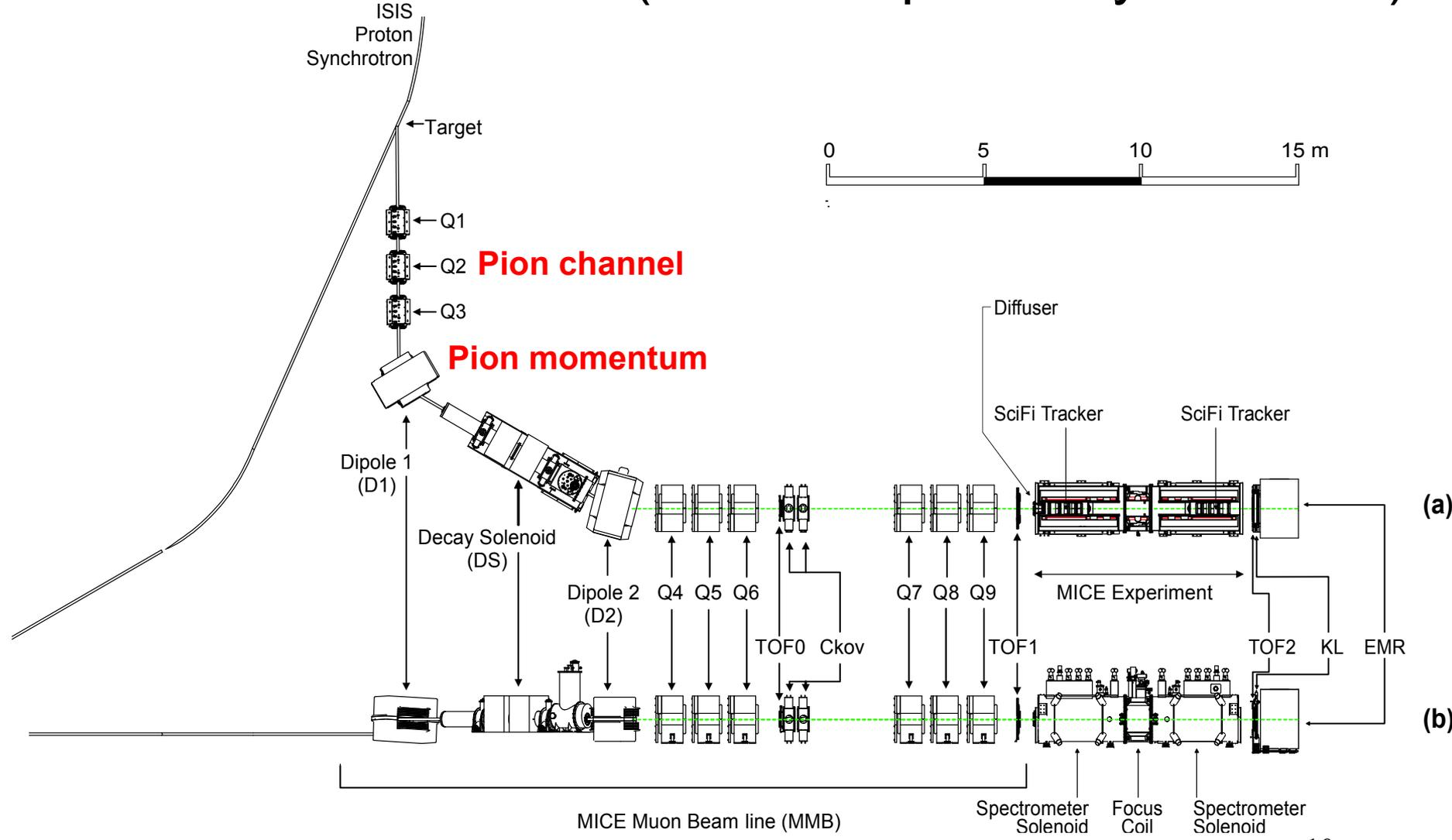
MICE Muon Beam line (MMB)
