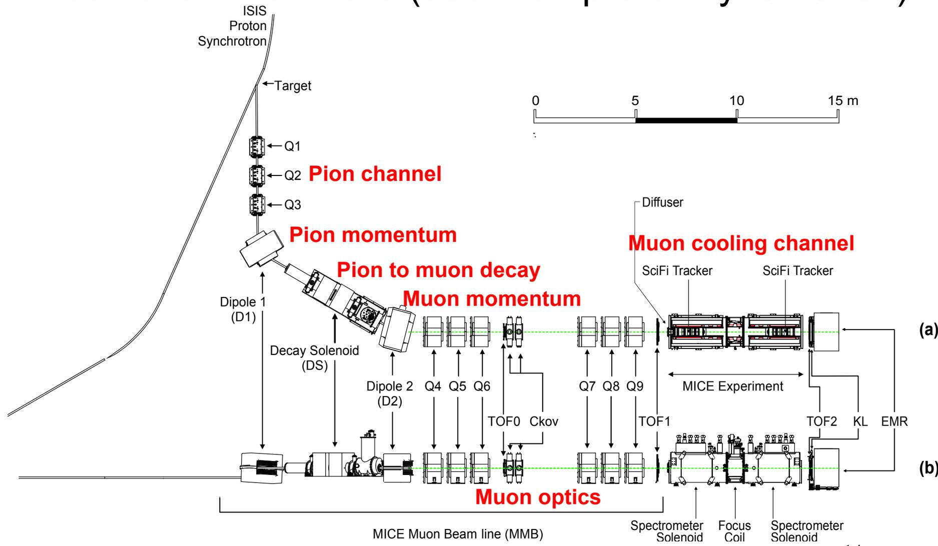
MICE Muon Beam line (MMB)
