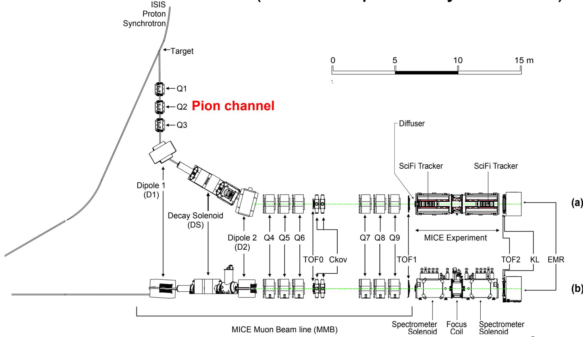
MICE Muon Beam line (MMB)
