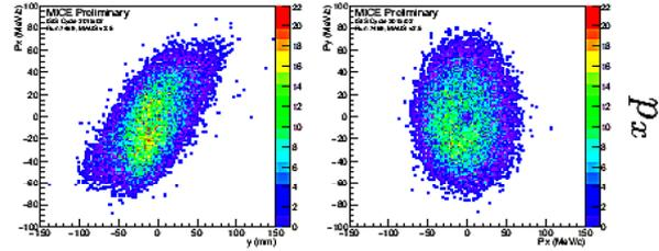
Ionization cooling implies reduction of transverse emittance after absorber
