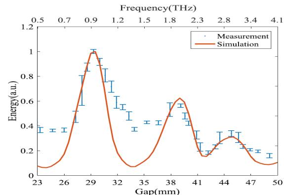
Measurement of pre-bunched beams' form factor based on radiation from a gap-tunable undulator
