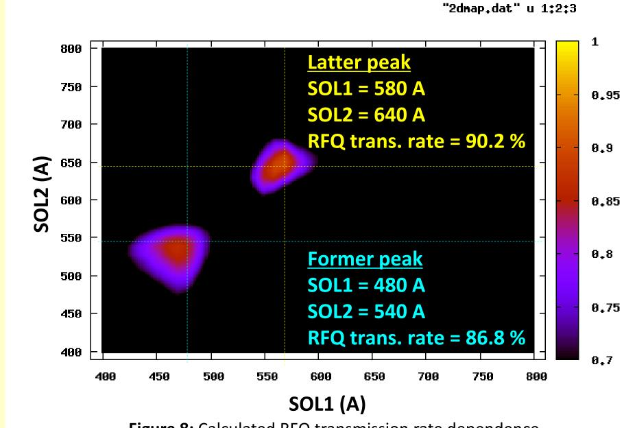
Figure 8: Calculated RFQ transmission rate dependence on the current settings of SOL1 and SOL2.
