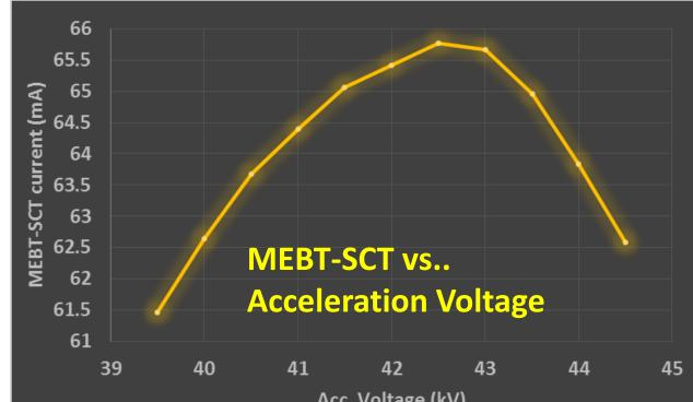
Figure 7: Dependence of MEBT-SCT current to the Acceleration Voltage in LI 60 mA operation.
