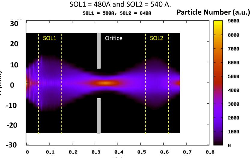
Figure 12: Calculated beam profile in the XZ plane for SOL1 = 580A and SOL2 = 640 A.
