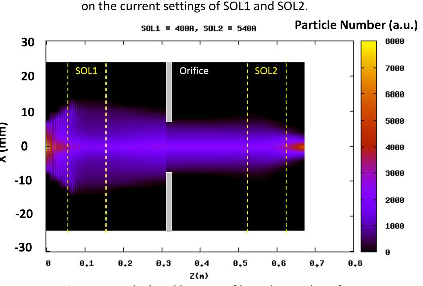
Figure 10: Calculated beam profile in the XZ plane for
