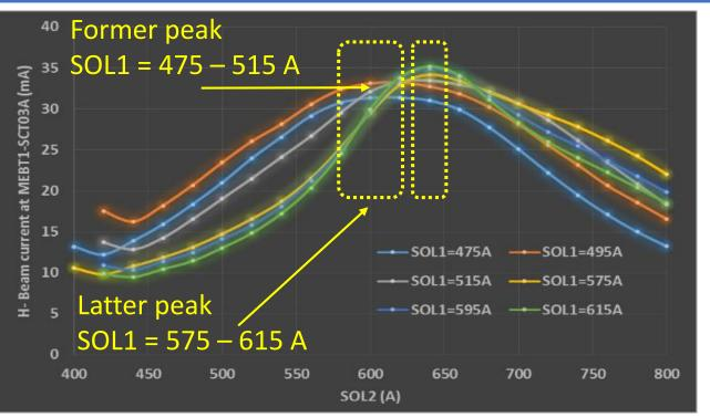
Figure 2: Dependence of MEBT-SCT current to the SOL1 and SOL2 currents in J-PARC Linac 30 mA operation.
