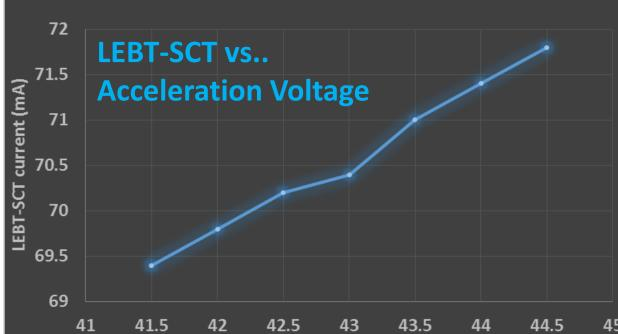
Figure 6: Dependence of LEBT-SCT current to the Acceleration Voltage in LI 60 mA operation.
