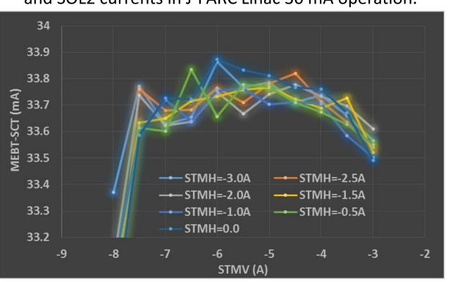
Figure 3: Dependence of MEBT-SCT current to the horizontal and vertical STM currents in LI 30 mA operation.
