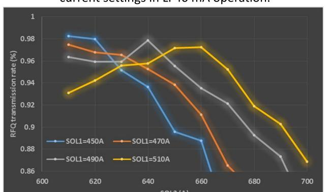
Figure 5: Dependence of RFQ transmission rate to the SOL1&2 current settings in LI 40 mA operation.
