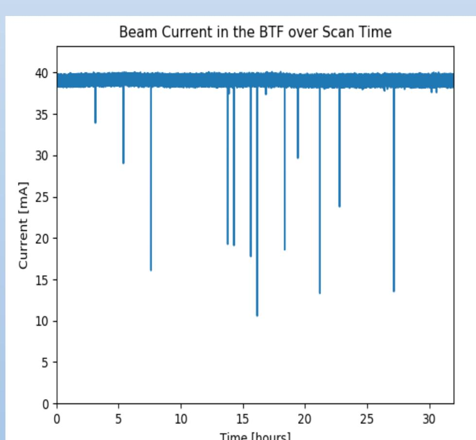
The SNS accelerator is very stable and quickly recovers from trips. This BTF is a function duplicate of the SNS Front End so it also retains these qualities.
