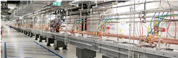
Figure 2: C-band accelerating structures in a part of the Linac 3.
