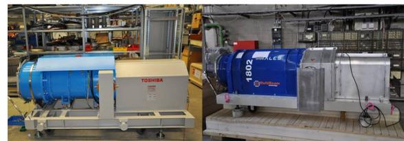
Figure 5: Multi beam klystrons for the E-XFEL.
