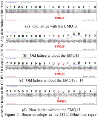
(d) New lattice without the EMO13 Figure 5: Beam envelope in the DTL1(Blue line represents horizontal envelope, red line represent vertical envelope, green line represent longitudinal phase width).
