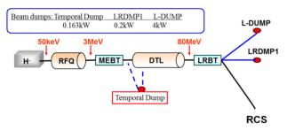
Figure 1: CSNS Linac layout.
