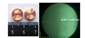
Figure 10: On the left – cavities, on the right – depiction of the aperture obtained with help of microscope.
