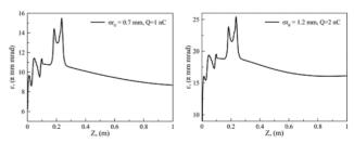
Figure 2: Emittance evolution for the beam from the photocathode gun with the charge of 1 nC (top) and 2 nC (bottom).
