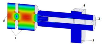
Figure 1: Layout of the photocathode gun with the electric field distribution: 1 - accelerating cavities, 2 - input for the laser beam, 3 - RF power input, 4 - vacuum pumping connection, 5 - photocathode.
