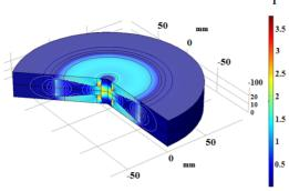
Figure 7: Magnet module with field lines.
