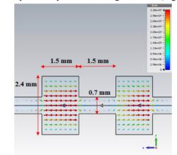
Figure 4: Two cavities of the excited W-band structure by the beam with  $\sigma_t = 2ps$ , Q = 2 nC.
