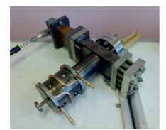
Figure 3: Fabricated photocathode RF gun.
