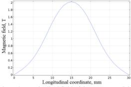
Figure 8: Longitudinal field of the magnet module.
