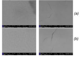
Figure 7: SEM images of HIPIMS samples. (a)~(b) the voltage of the laser (power density) is from 14kV to 16kV (exposure time is 30s). Different columns represent different magnification ( $\times$  1k and  $\times$  50k).
