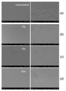
Figure 8: SEM images of HIPIMS samples before and after annealed. There are few cracks and the length of a crack decreases to several hundred nm. (a) Unannealed Nb/Cu film; (b) $\sim$ (d) The exposure time increased from 10s to 30s, 60s (voltage is 13.5kV). Different columns represent different magnification ( $\times$  1k and  $\times$  50k).
