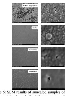
Figure 6: SEM results of annealed samples of dcMS. The voltage of the laser (reflect the power density) is 14kV. Different columns represent different magnification (× 1k and × 80k). With the laser exposure times increased (5s/1Hz, 1~2s/5Hz, 10s/1Hz, 20s/1Hz), the cracks increase too. The film grains melt, and grain boundaries and fade away.
