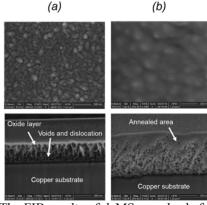
Figure 5: The FIB results of dcMS samples before(a) and after(b) annealed. It can be observed that defects decrease a lot, but the annealing is not very uniform.
