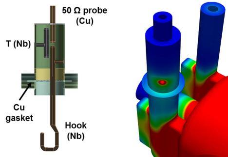
Figure 10: Cu gasket location at the HHOM coupler (left) and rf losses at the stainless steel flange (right).
