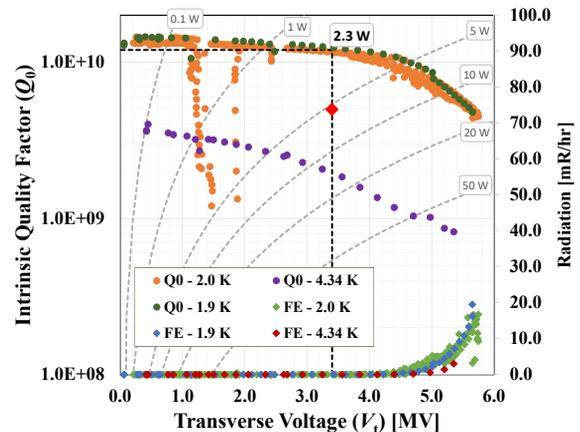
Figure 3:  $Q$  curves of the bare RFD-CAV-002.
