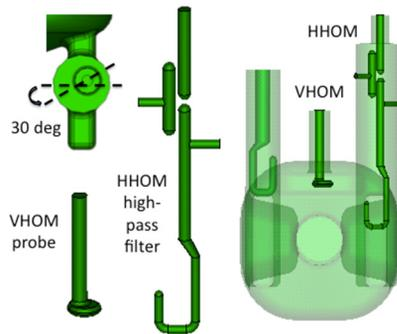
Figure 4: HHOM and VHOM couplers for the rf-dipole crabbing cavity.
