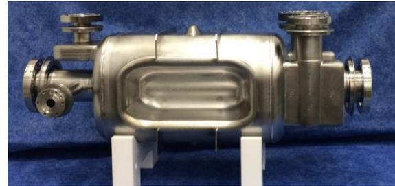
Figure 2: Fabricated Nb rf-dipole cavity.
