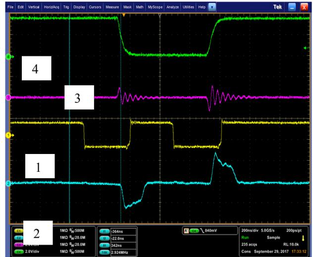
Figure 2: Signals of integrate and hold circuit. Channel 1 is the charge reset signal (active high), channel 2 is integrator output, channel 3 is the current monitor output from HC switch, and channel 4 is the voltage monitor output.
