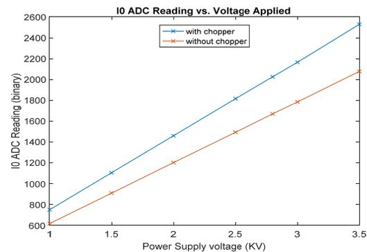
Figure 3: ADC reading of integrated charge/discharge current versus high voltage applied to the capacitor load of HV switch, with and without chopper (with  $C_{cable}$  and  $C_{sw}$  only).
