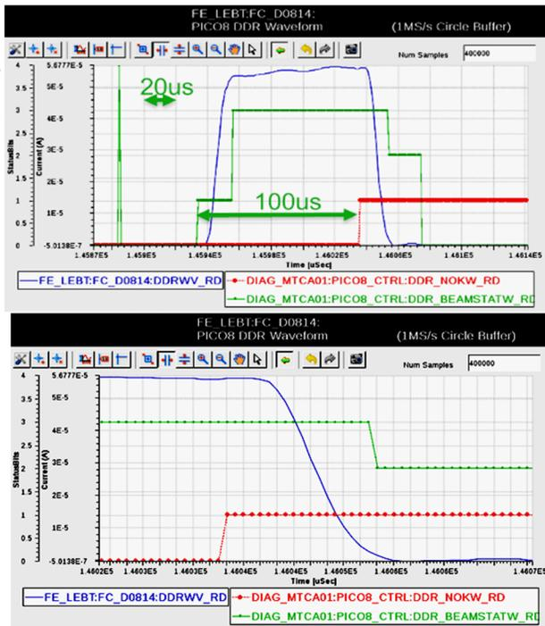
Figure 4: State transitions immediately following the request for 120  $\mu\text{s}$  pulse duration. Top display: the chopper monitor detects a beam-on condition (green) persisting longer than authorized, initiating the MPS NPERMIT response (red). Bottom display: expanded view of Faraday cup beam current signal.
