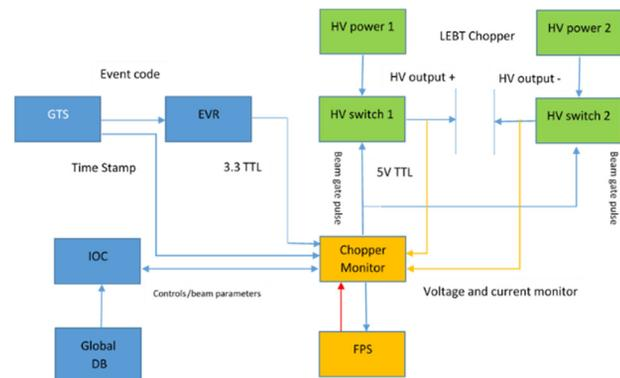
Figure 1: FRIB Chopper Control and Monitor System block diagram.
