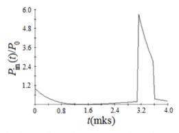
Figure 3: The envelope of RF power coming to input of the accelerating structure after the SLED system.
