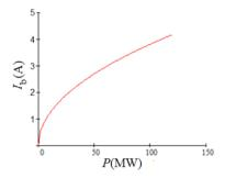
Figure 2: Critical beam current which can pass through structure at a zero gradient of a field in a stationary regime.
