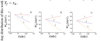
Figure 5: Full energies received by a beam in the accelerating structure for different RF power of the generator and different beam currents: a - TH2129 + SLED, b - E3730A + SLED, c - 5045 SLAC + SLED,  $1 - I_b = 1 \text{ A}, 2 - I_b = 2 \text{ A}, 3 - I_b = 3 \text{ A}.$
