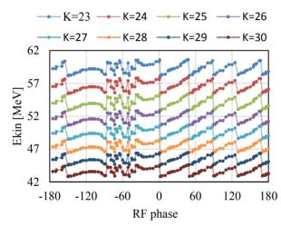
Figure 5: CCDTL1 phase scan: single BPM pair with different K values.
