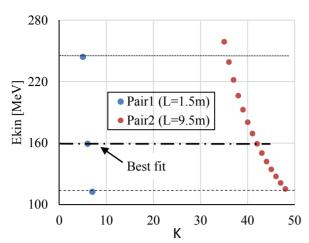
Figure 4: Single energy ToF measurement using 2 BPM pairs.
