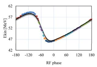
Figure 6: CCDTL1 RF phase scan cleaned after fitting. Simulated data as black crosses.
