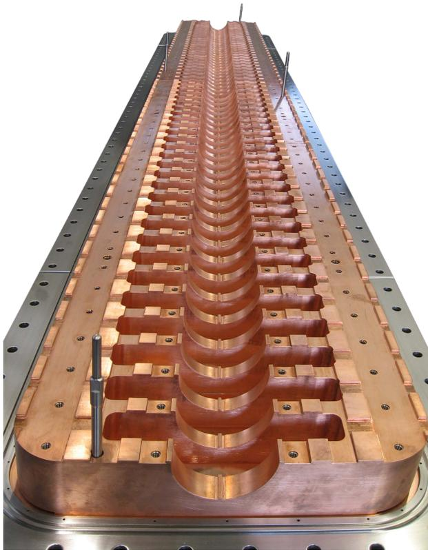
Figure 2: Lower half-ladder structure after finalization of surface treatment and assembly on the lower tank shell.
