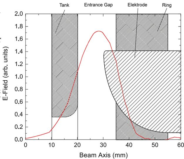
Figure 5: Longitudinal fringe field in the entrance gap/radial matching section of the RFQ.
