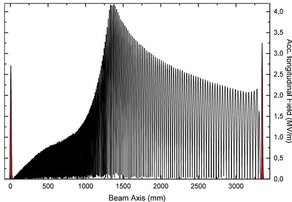
Figure 6: Longitudinal electric field on the beam axis. Simulation result of a complete 3D EM eigenmode simulation considering the entire final modulation of the electrodes. The entrance and exit fields are colored in red.
