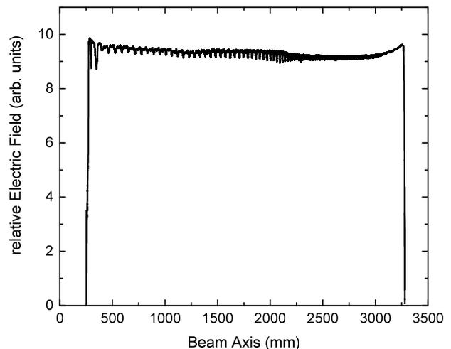
Figure 4: Field flatness of the Ladder-RFQ along the beam axis before tuning procedures.
