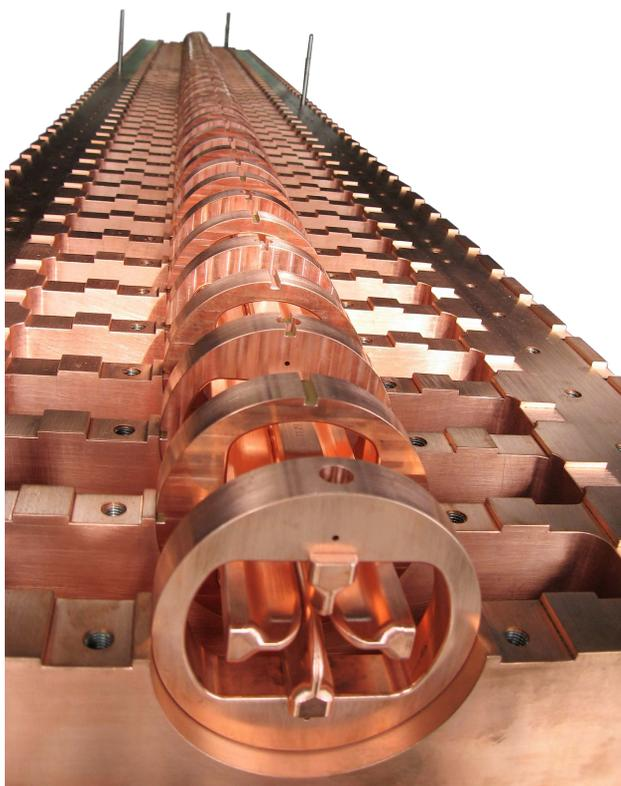
Figure 3: Assembly of the electrodes and carrier rings.
