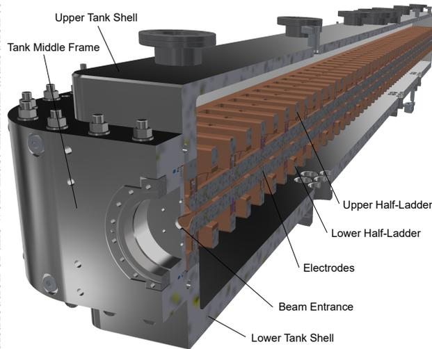
Figure 1: Isometric view of the 3.3 m modulated Ladder-RFQ. Copper carrier-rings guarantee the electrode positioning as well as the RF contact. The ladder structure consists of bulk copper components. Any brazing or welding processes were avoided for the assembly of the main components.
