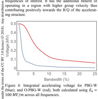
Figure 4: Integrated accelerating voltage for PBG-W (blue), and O-PBG-W (red), both calculated using  $E_0 =$ 100 MV/m across all frequencies.
