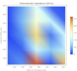
Figure 2: Variation of characteristic impedance with PBG-W thickness and channel width.
