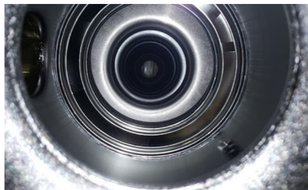
Figure 7: No grinding marks after BCP.
