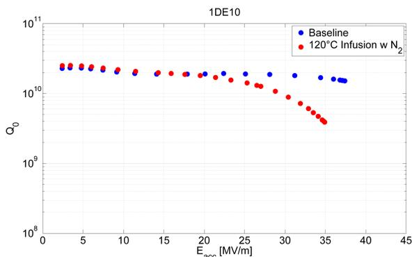
Figure 6: Quality factor versus accelerating field of 1DE10 before (blue) and after the treatment (red).
