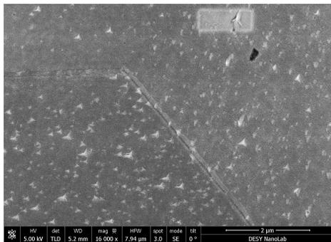
Figure 10: SEM image of a cut out from 1DE16. The same star shaped precipitates are observed as on the sample inside the Nb box.
