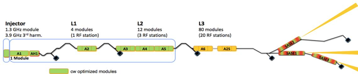
Figure 1: The first 17 modules (136 cavities) of the European XFEL need to be replaced to achieve the desired flexibility for the user operation. An SRF gun based cw injector and one IOT for each rf station is necessary. L3 remains unchanged.
