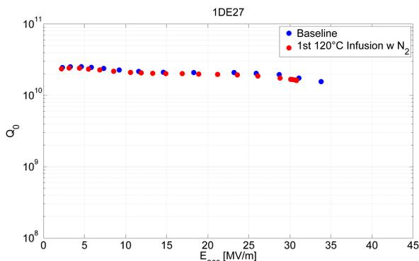
Figure 7: Quality factor versus accelerating field of 1DE27 before (blue) and after the treatment (red).
