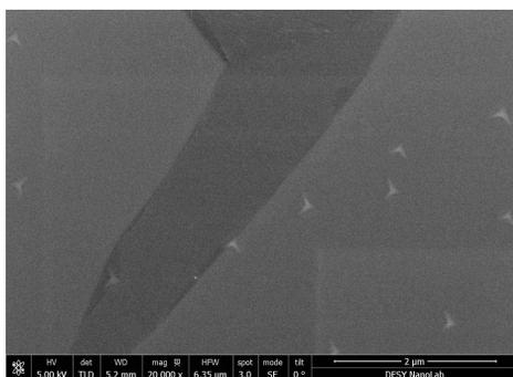
Figure 11: SEM image of a cavity-grade single-crystal sample after baking in an ultra-clean chamber. Similar star-shaped precipitates as on the cavity furnace samples can be seen. No precipitates were observed on the purified sample.
