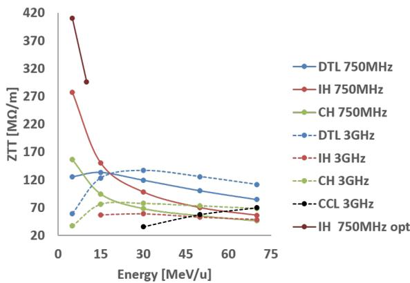
Figure 2: ZTT as a function of the RF cavity energy for different low energy RF cavities [12].
