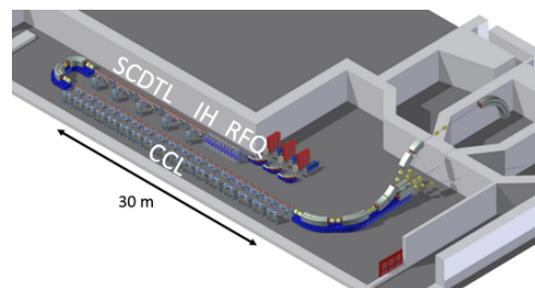
Figure 5: Sketch of CABOTO all-linac solution (courtesy of M. Vaziri—TERA Foundation)
