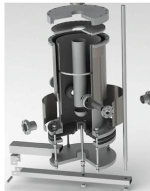
Figure 7: General view of 162 MHz QWR design model.
