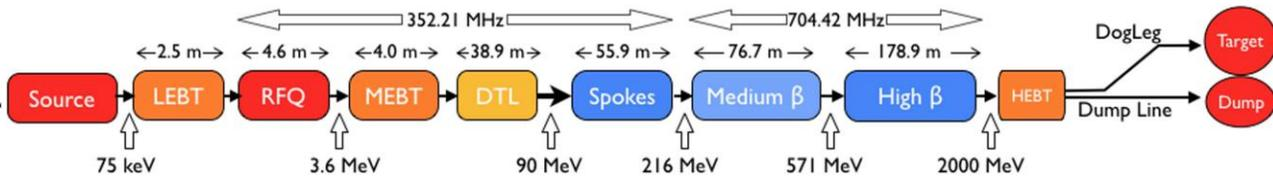
Figure 2: ESS Linac lattice overview.
