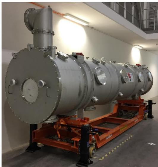
Figure 3: Cryomodule for installation tests at ESS.
