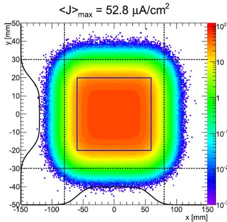
Figure 5: The intensity profile across the target after raster scanning. Note 3:1 aspect ratio on scales.
