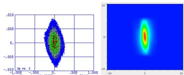
Figure 10: Simulated and measured emittance in y-direction in MEBT.
