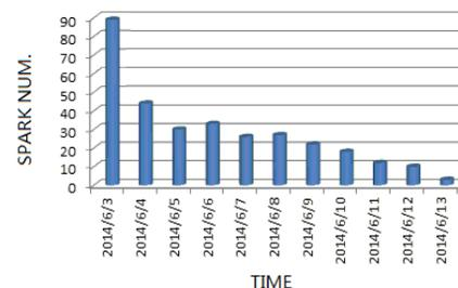
Figure 7: Spark number of RFQ cavity declined during high-power conditioning of 11 days.
