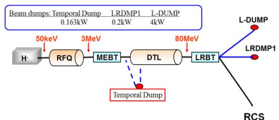
Figure 4: Linac beam dumps for beam commissioning.
