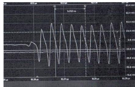
Figure 6: Measured beam rise time about 10ns after LEBT chopper.
