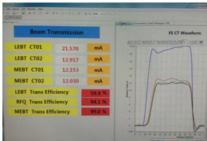
Figure 8: The best beam transmission rate of the RFQ.
