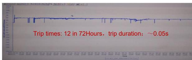
Figure 5: Record of the ion source trip rate in 72 Hours after improvement.
