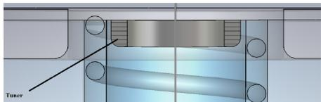
Figure 4: Frequency adjuster tuner core.
