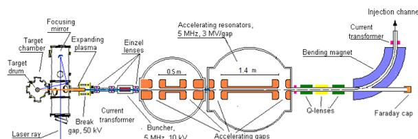
Figure 2: Acceleration structure of I-3M.
