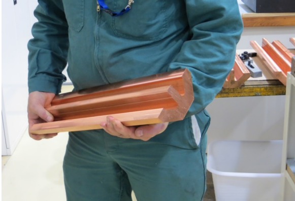
Major vane after final machining
