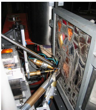
Stained glass panel analysed by PIXE/PIGE/RBS with 3-MeV protons
