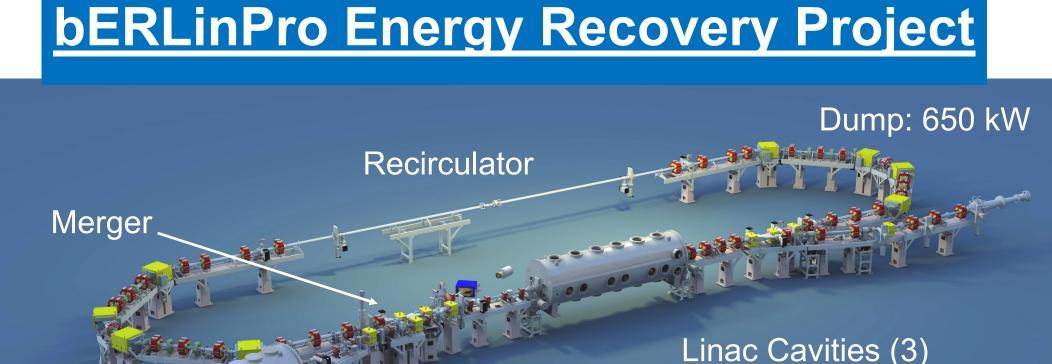
**bERLinPro's** main **goal** is the ERL operation of a low emittance, high current beam  $(\varepsilon_n < 1 \text{ mm mrad}, I_{beam} = 100 \text{ mA}, \sigma_t = 2 \text{ ps}).$ Its basic concept starts with a 6.5 MeV injector consisting of a 1.4<sup>- $\lambda$ </sup>/2 cell SRF gun followed by a booster section with three 2-cell-cavities.
