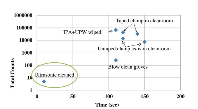
**Surface particle count is material dependent and surface finish** dependent. Metal is easier to blow clean than plastic. Polished surface is easier to blow clean than rough surface.
