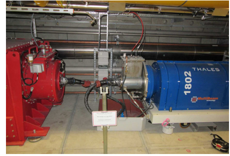
HV connection between pulse transformer and MBK
