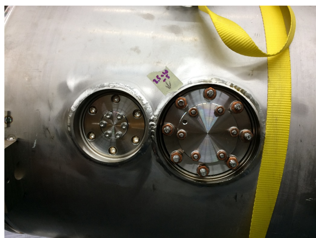
Position of the leak (coupler port).
