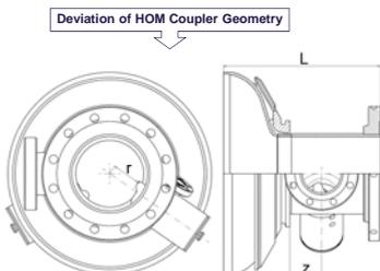
Figure 2: Position of High Order Modes (HOM) coupler #1 in the short end group (EGS):
