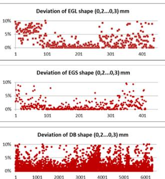
Figure 5: Part of subcomponents shape with accuracy deviation over 0.2 nm.
