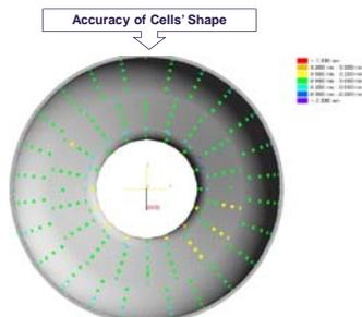
Figure 4: Results of 3D-measurements of cavity half-cell.
