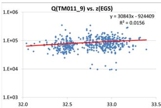
Figure 3: Sensitivities of quality factor for TM011 (y) to EGS geometry deviations (x = L, z and r) in mm.
