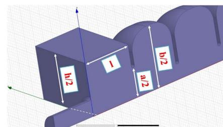
Layout of an electric-coupled RF coupler
