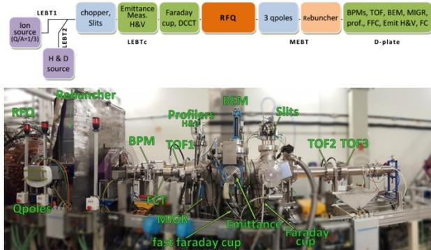
Figure 7: Injector scheme and Diagnostic Plate picture.
