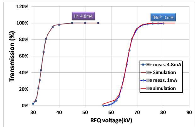
Figure 9: Comparison between measurement and TraceWin/Toutatis simulation (p and He beams).
