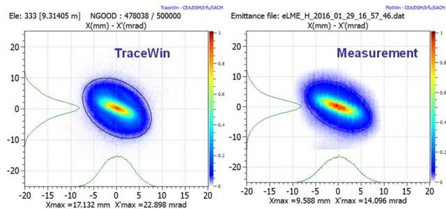
Figure 10: 5 mA proton beam in the D-plate.
