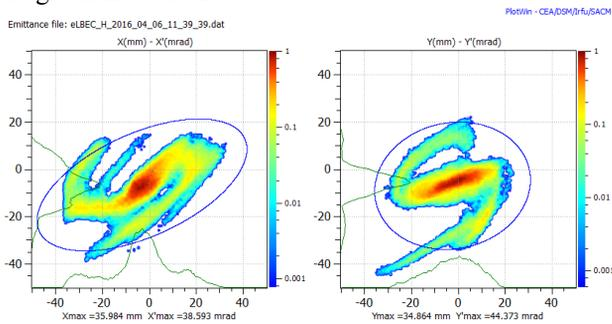
Figure 4: LEBTc emittance measurement for a 1.35 mA He beam, open slits, before hexapole tuning optimization.
