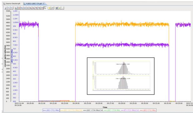
Figure 8: 4.8 mA proton beam current measured before (orange) and after (magenta) the RFQ. The 2 curves superimposed at both ends show the 100% transmission. In the middle, a profiler inserted just after the RFQ intercepts a part of the accelerated beam.
