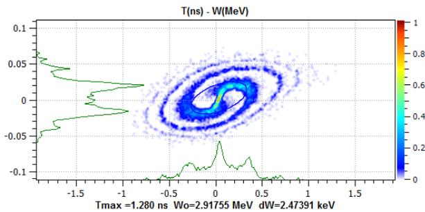
Figure 13: TraceWin simulation of a 0.15mA He beam at the BEM location.
