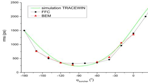
Figure 11: Comparison of the bunch width between FFC, BEM and TraceWin simulations.
