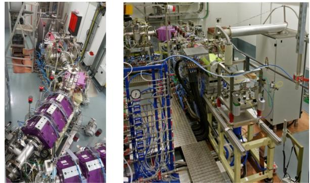
Figure 1: sources and LEBT at GANIL/SPIRAL2. Left : light ion source (H<sup>+</sup>, D<sup>+</sup>), right : heavy ions (Q/A=1/3).
