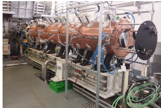
Figure 5: RFQ during the bead pull measurement.
