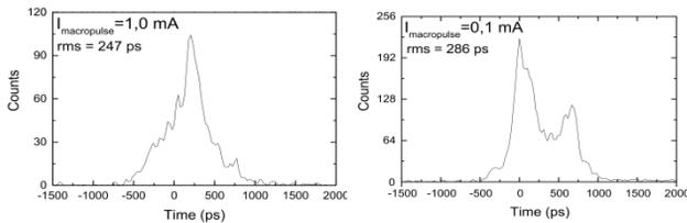
Figure 12:  $^4\text{He}^{2+}$  longitudinal bunch shape for 1 and 0.1 mA.
