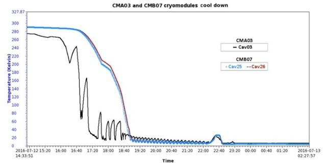
Figure 14: Very first cool down of linac cryomodules.
