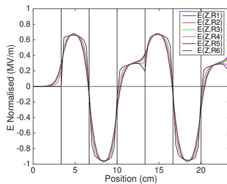
Figure 3: Longitudinal fields at subsequent radii cross the bore tube and first six cells.
