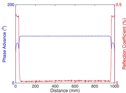
Figure 1: a) A CST drawing of the 30 cell linac with couplers. b) Evolution of phase advance and the reflection coefficient along the linac.
