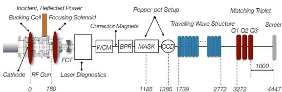
Figure 2: Layout with AWAKE e<sup>-</sup> injector.
