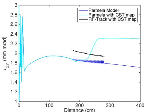
Figure 4: Tracking results for emittance evolution along the beamline.
