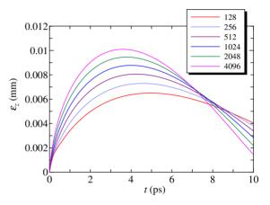
Figure 7: Time evolutions of rms emittance with 4096, 2048, 1024, 512, 256 and 128 macro particles.
