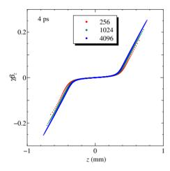
Figure 5: Phase space distributions at t = 4 ps. The number of macro particles are 4096, 1024 and 256.
