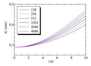
Figure 6: Time evolutions of bunch length with 4096, 2048, 1024, 512, 256 and 128 macro particles.
