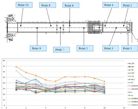
Figure 4: WIC thickness measurement example.
