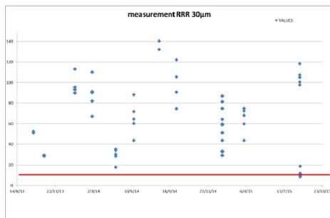
Figure 8: RRR dispersion on copper coating at 30  $\mu\text{m}$ .
