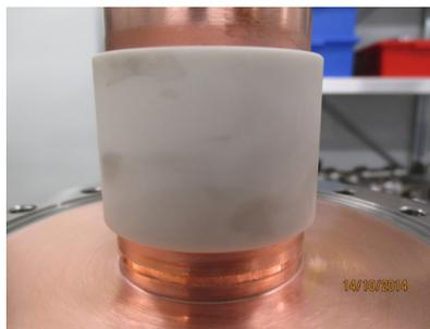
Figure 9: Tinted ceramic after RF conditioning.
