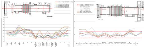
Figure 3: WEC, CEC thickness measurements example.
