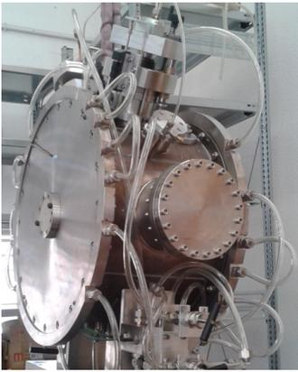
Figure 2: Picture of one of the re-buncher cavities.
