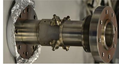
Figure 4: Picture of one of the vacuum chambers including a beam position monitor.
