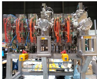
Figure 7: MEBT assembled at CIEMAT.
