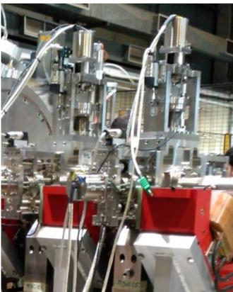
Figure 3: Picture of the scrapers installed in the beamline with the magnets opened.
