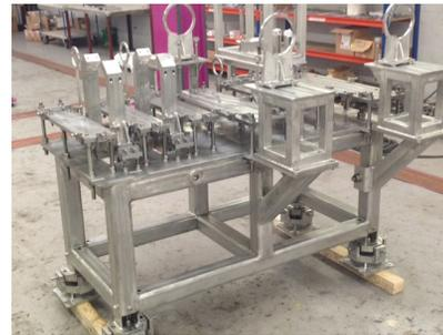
Figure 5: Picture of the mechanical frame for the MEBT with the alignment supports for individual components.
