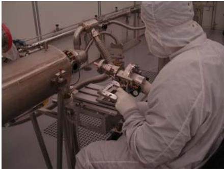
Figure 4: Cold end coupler assembly.
