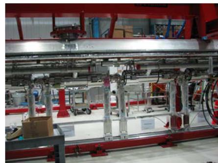
Figure 8: Upper cold mass to cavity string assembly.
