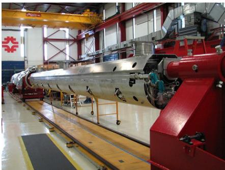
Figure 10: Cold Mass Assembly at WS4.
