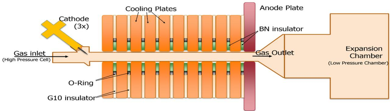
Figure 1: Schematic (not to scale) of the Plasma Window. Ten cascaded arc cooling plates of floating potential are each 1 cm in width and separated by 1mm of O-ring, boron-nitride spacers, and G10 spacers to insulate them from their neighbors. Three thoriated tungsten needle cathodes collectively deliver up to 90 amps.
