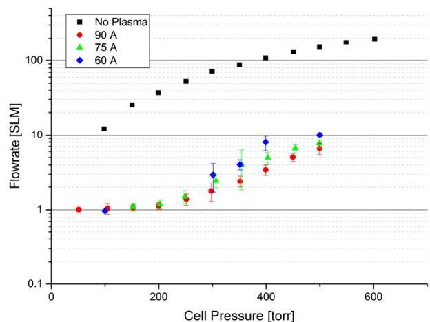
Figure 2: Flowrate values for both un-ionized gas flow and plasma at multiple current values. Error bars are the standard deviation of all points (between 50 and 150 points) during the collection time for a specific pressure setpoint.
