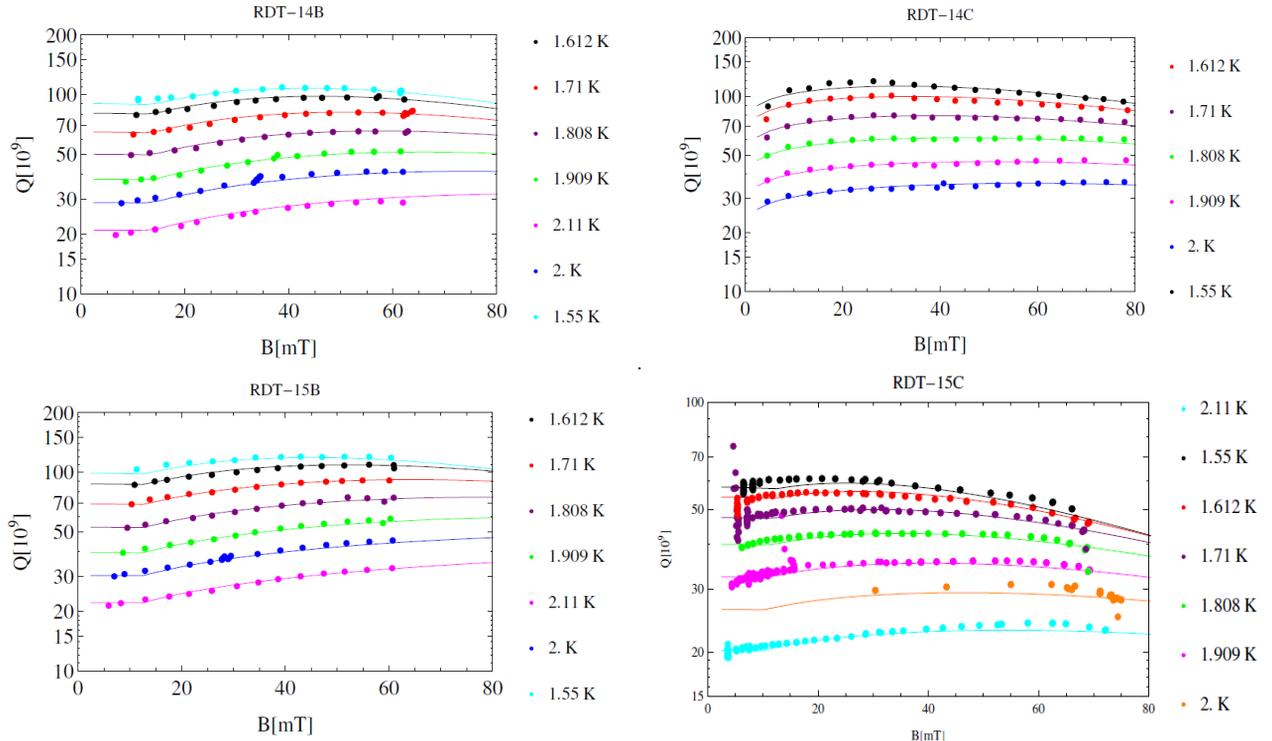
Figure 2: Q values versus peak magnetic surface field for the 4 cavities under study.
