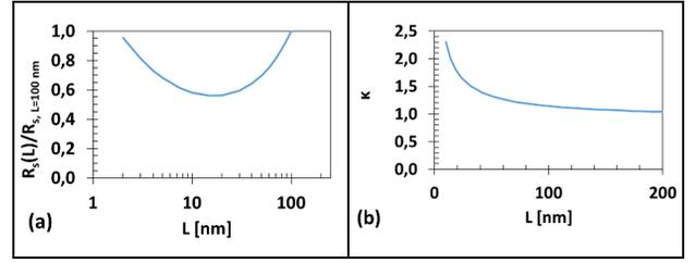
Figure 1: Dependence on L of (a) the ratio of  $R_s$  at B-field optimum and low B and of (b) the Ginzburg-Landau parameter  $\kappa$ .
